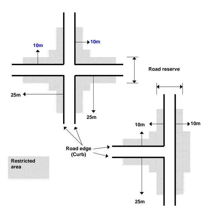
Figure 3: Additional restriction on illuminated signs at signalized street corners
