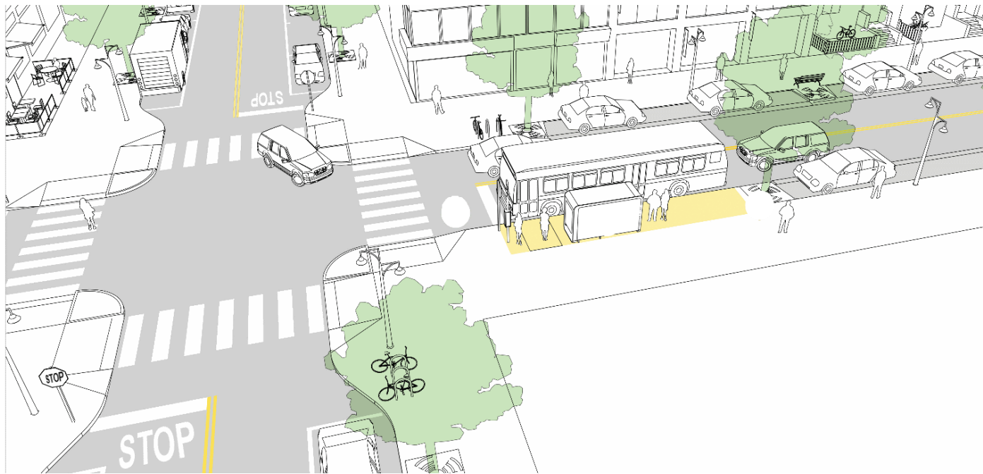
Figure 2-9: Near-Side Uncontrolled Station -Bus Stop In Lane
