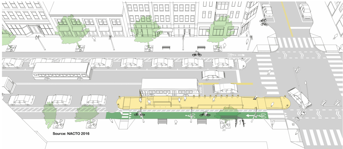
Figure 2-8: Far-Side Large Stations -Bus Stop In Lane
