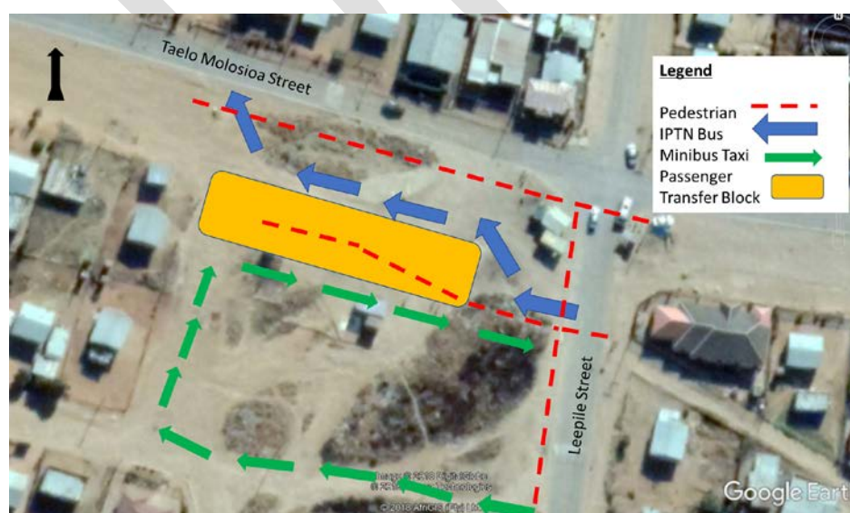
Figure 14: Concept Layout of Oliver Tambo Route Turnaround/Transfer facility
