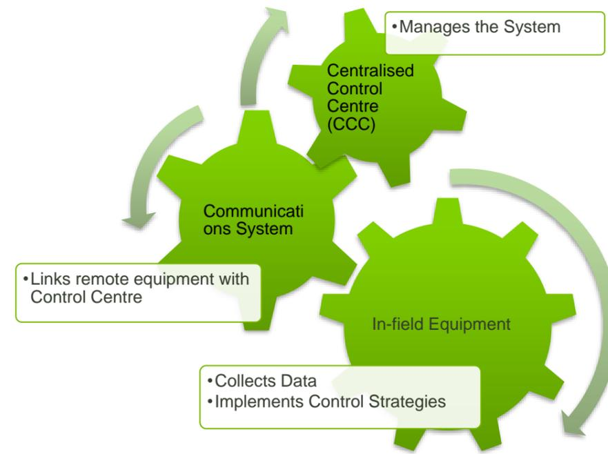
**Figure 14-25: Typical ITS Technology Modules**
