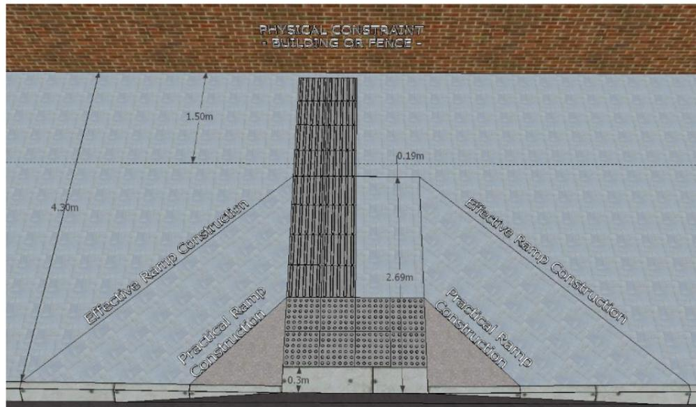
**Figure 14-26: Effective and Practical Ramp Construction**
