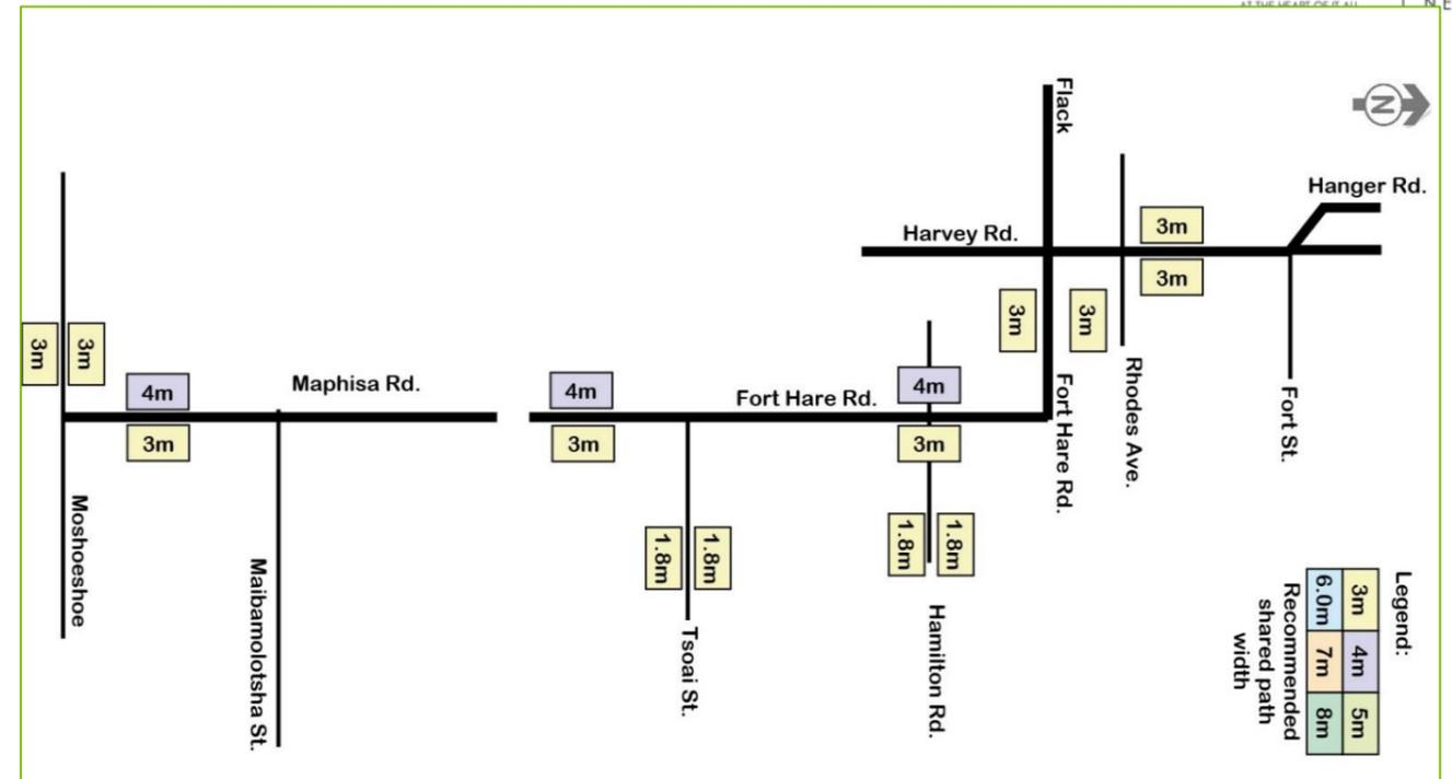
Figure 14-29: Recommended NMT Facility Widths
