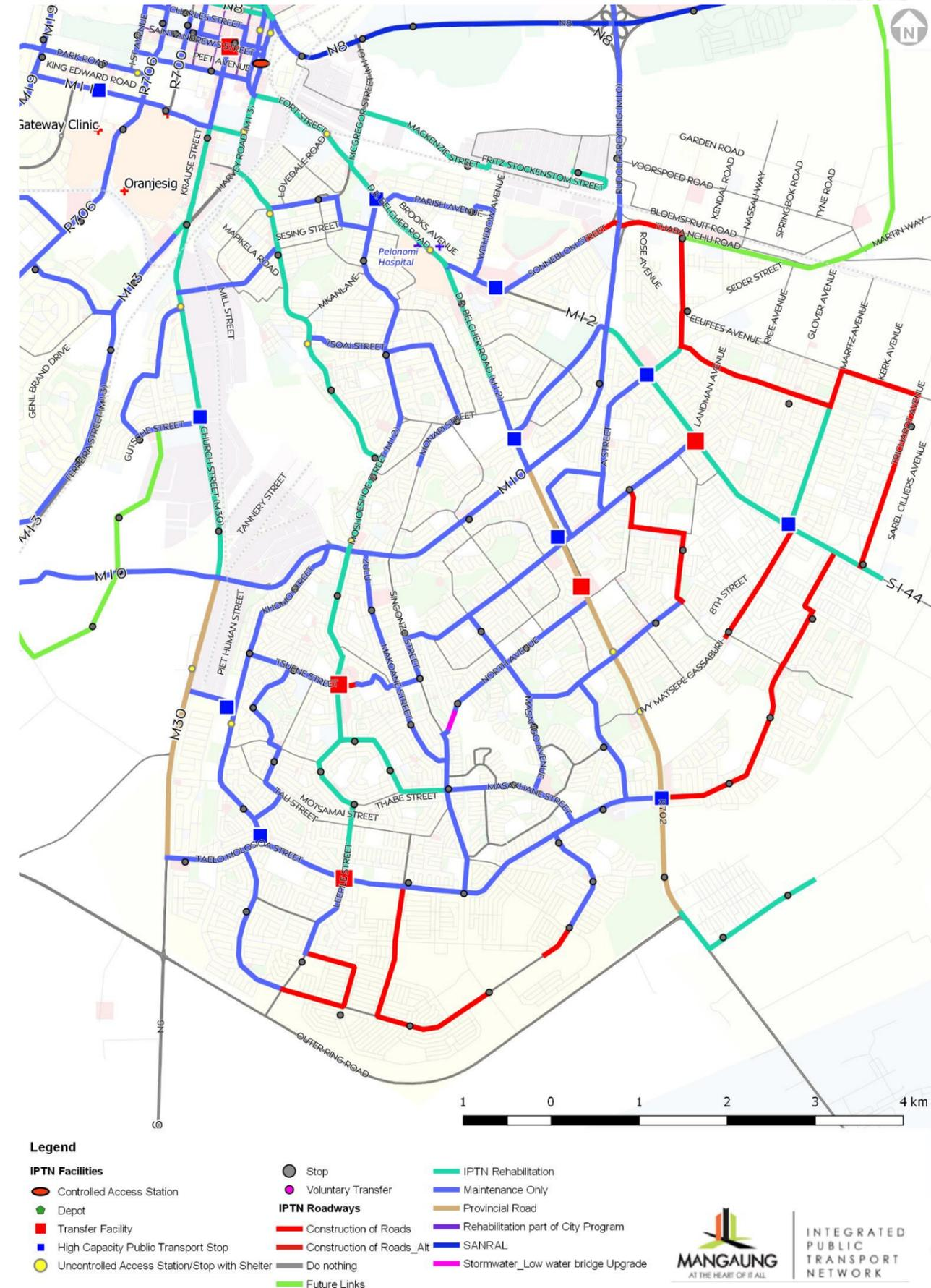
Figure 19-6: Roadway Upgrades and Maintenance Requirement South Eastern Quadrant
