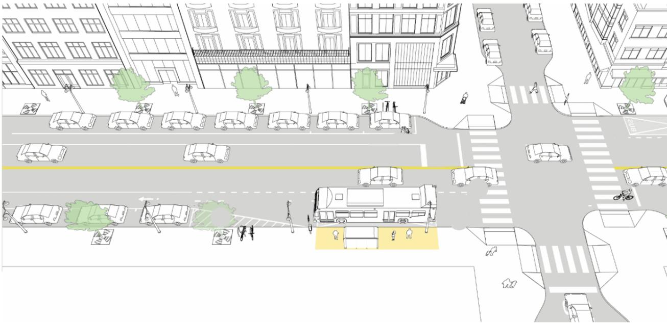
Figure 14-6: Far-Side-Uncontrolled Station-Bus Pull-Out
