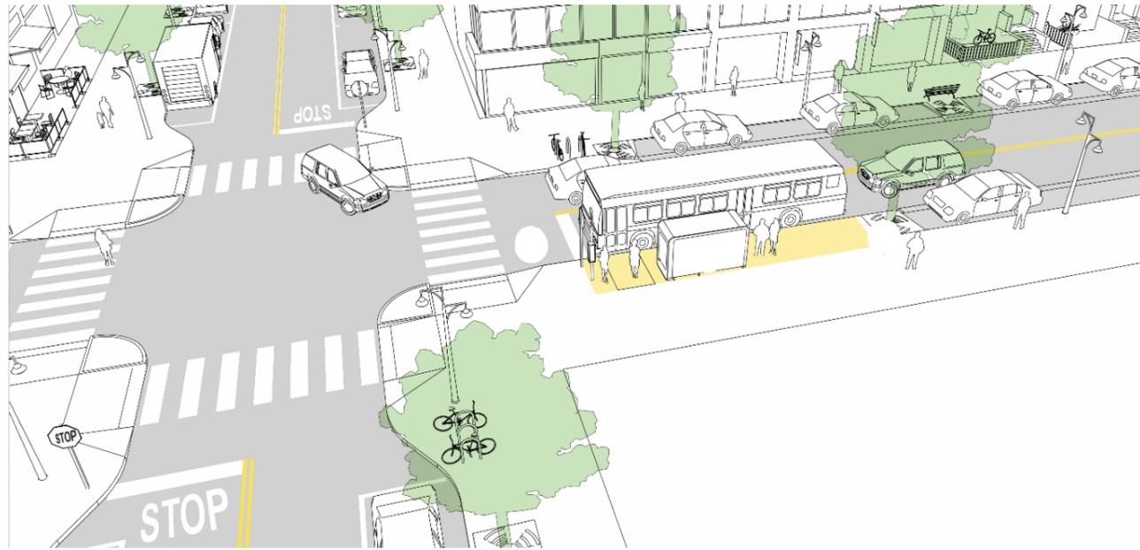
Figure 14-5: Near-Side Uncontrolled Station –Bus Stop in Lane
