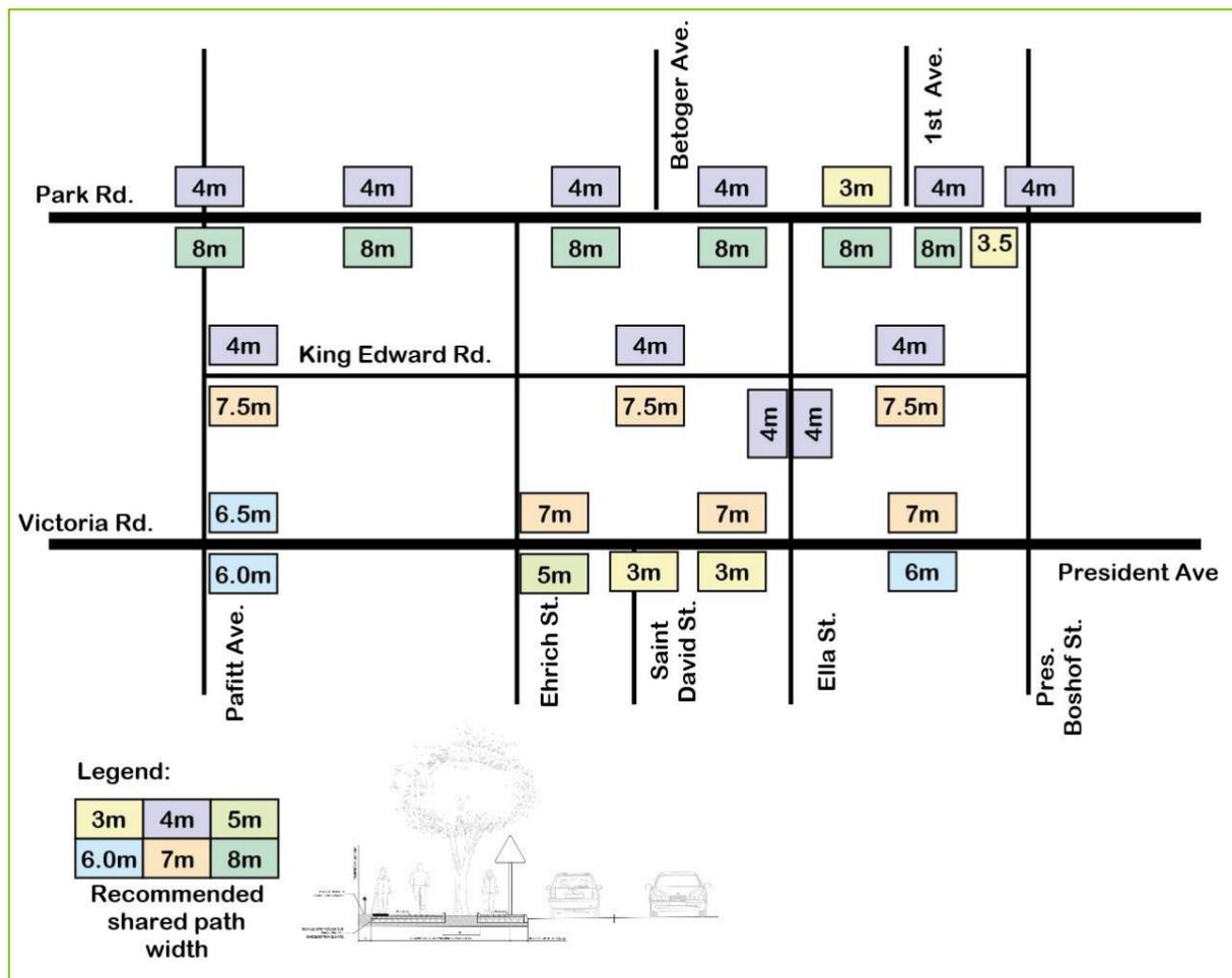
Figure 14-27: Recommended NMT Path Width
