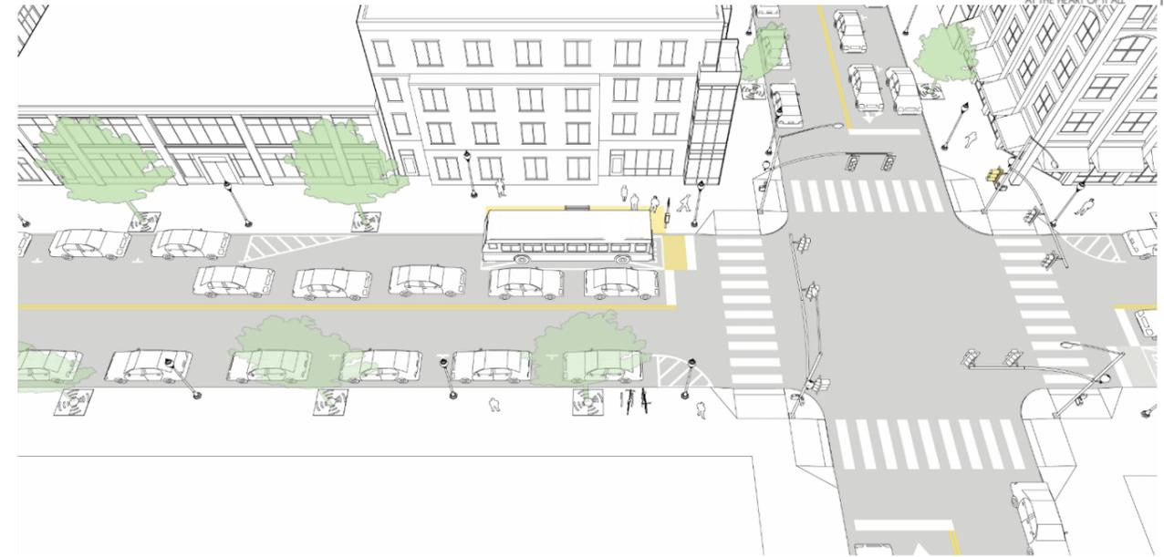
Figure 14-7: Near side – Uncontrolled Station (Queue Jump)
