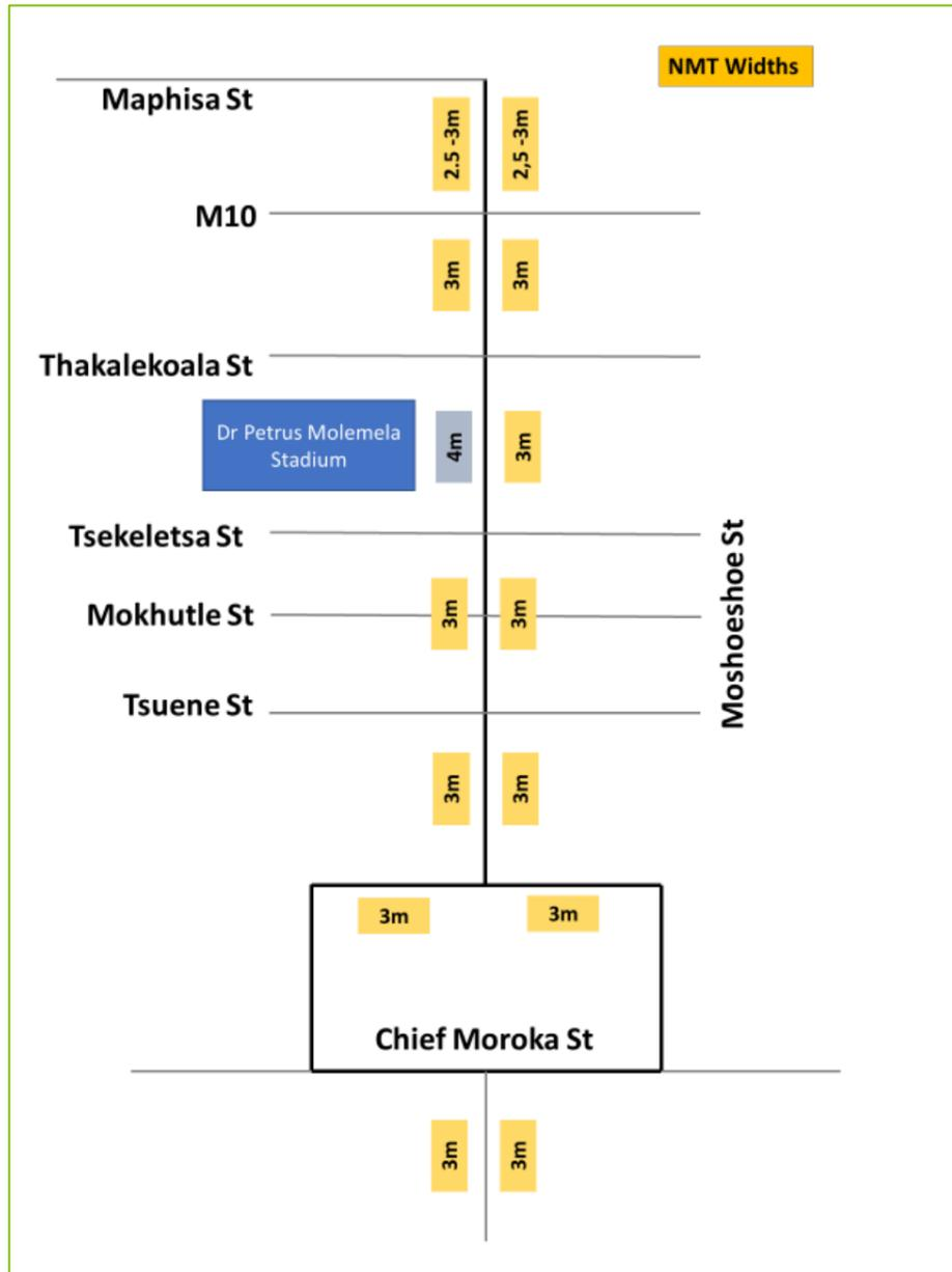
Figure 14-30: Recommended NMT Facility Widths
